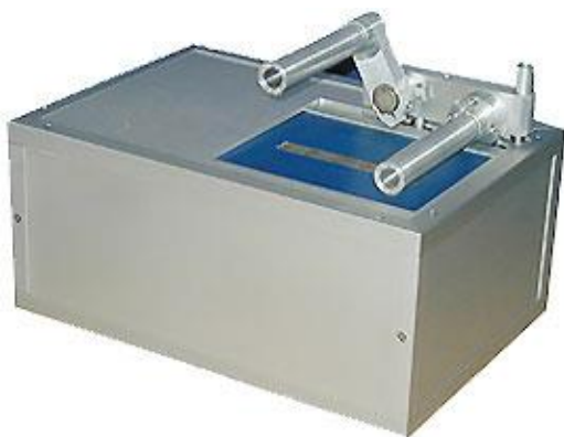
Fig. 9. 1-D surface NMR imager
